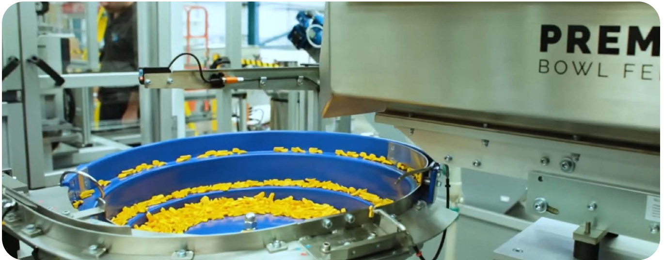
Bowl feed testing at PCE Automation
